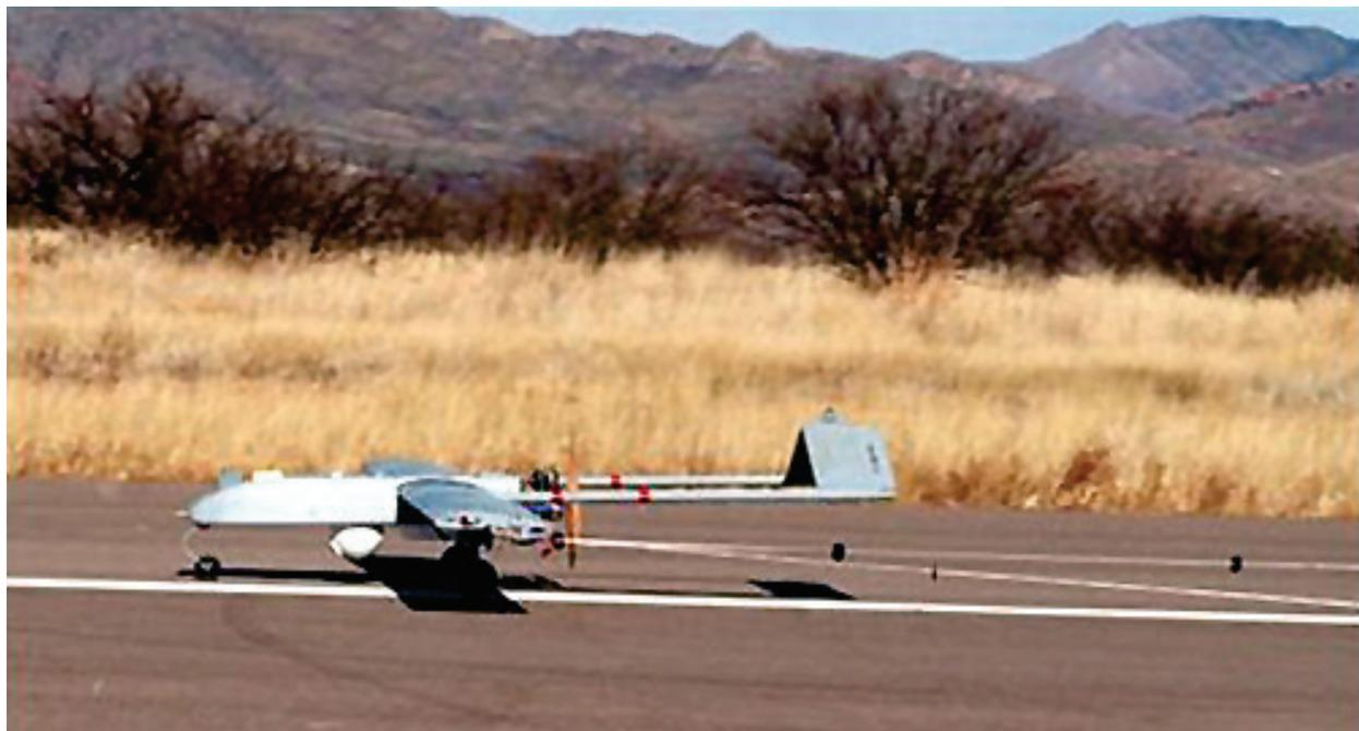
**Figure 1.3-1. RQ-7B Landing with Arresting Gear**
