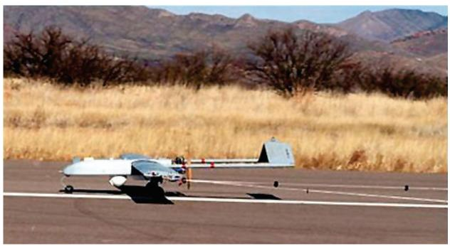
Figure 1.3-1. RQ-7B Landing with Arresting Gear
