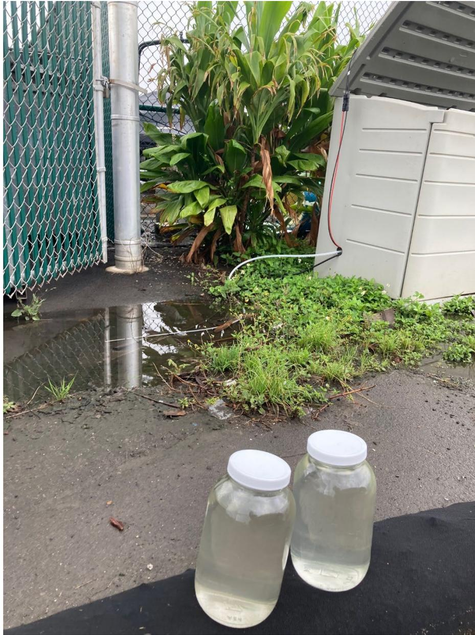
**Photo A-3. 2023 Q1 Benchmark samples in 2-liter glass sample jars at sample point**
