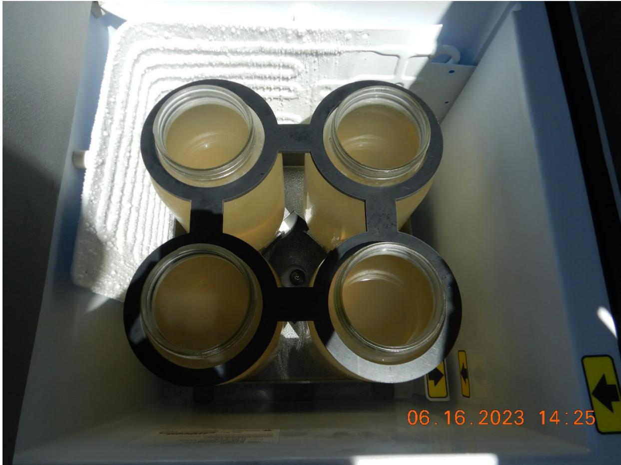
**Photo A-2. Sample jars in refrigerated autosampler at Building 132**
