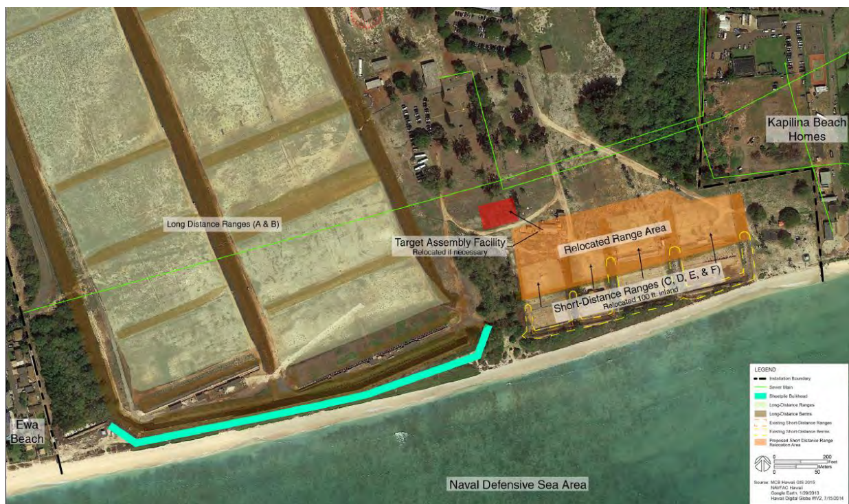
Figure 9. Sheet pile (depicted by the blue line) would be placed in front of the long-distance ranges (A, B), but not in front of the short-distance ranges. The four short-distance ranges (C-F) would be relocated back from the shoreline to the maximum extent practicable (possibly 100 feet back), since there is available land behind the ranges which would allow relocation. Revegetation would occur along and near all ranges, as feasible, in order to promote sand retention.
