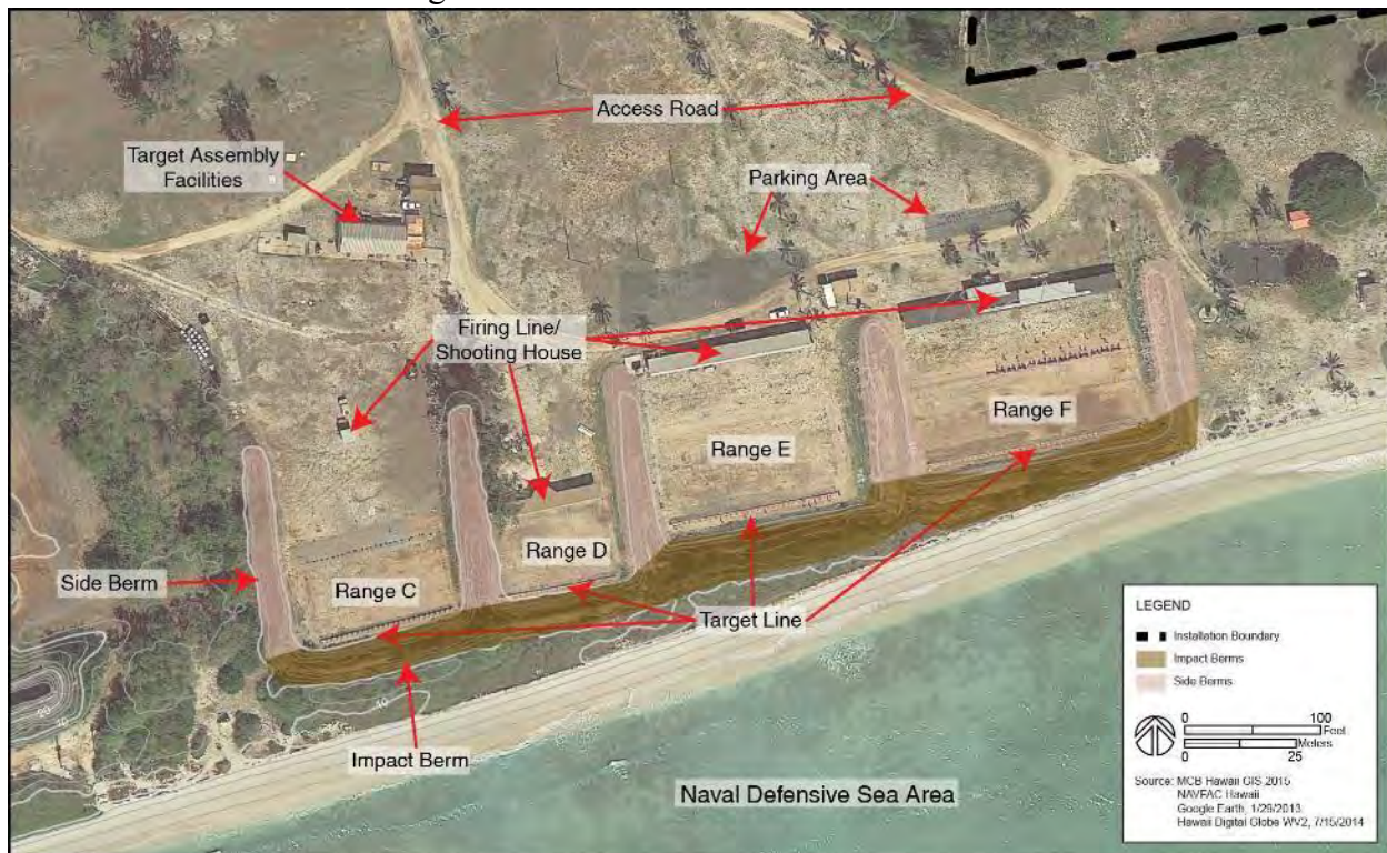
Figure 12. Berms fronting the short-distance ranges, and other components of the ranges shown would be relocated up to 100 feet back from the shoreline.
