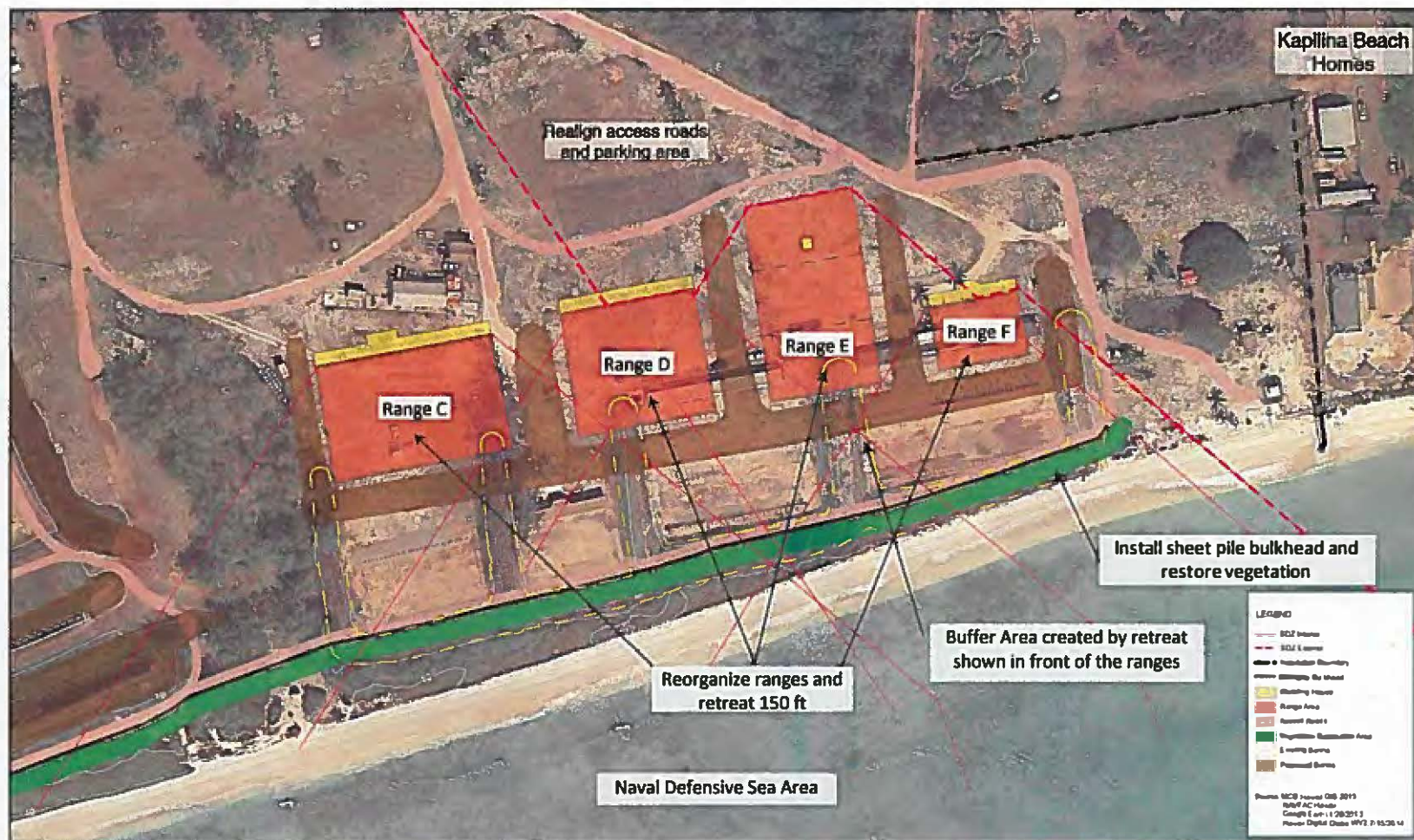
Puuloa Range Training Facility Shoreline Stabilization EA Reconfigure Ranges with a Maximum Retreat (150 ft.)
