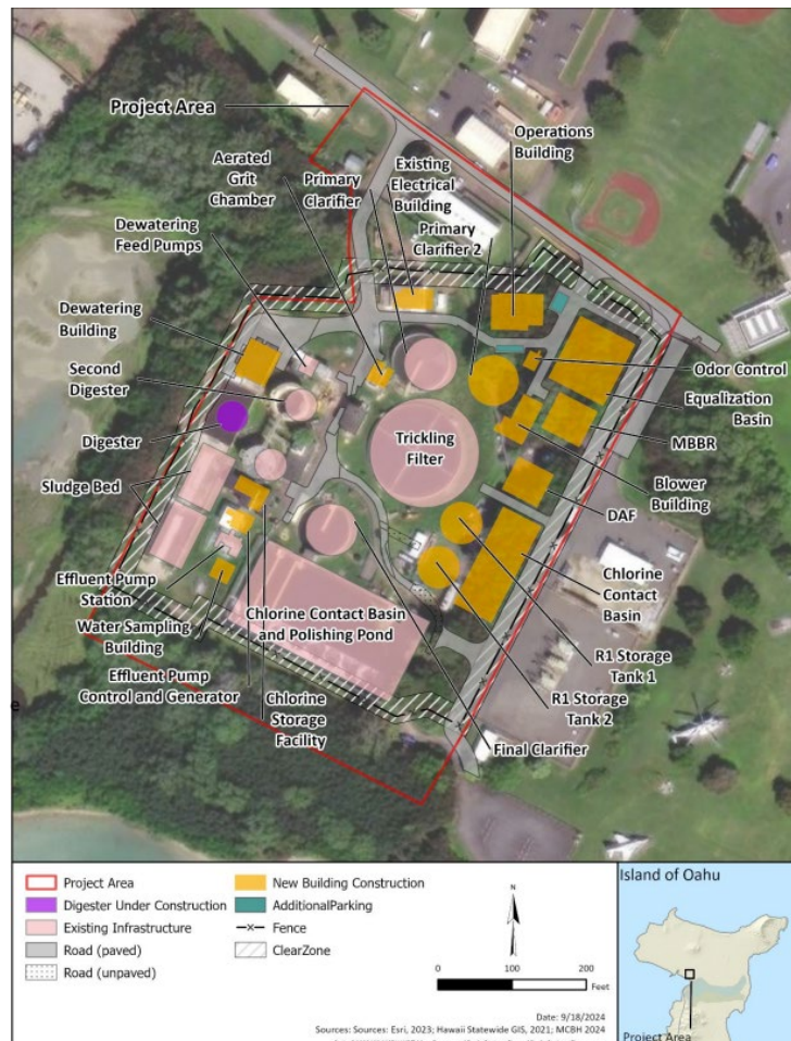
Figure 1. Proposed Water Reclamation Facility Upgrade
