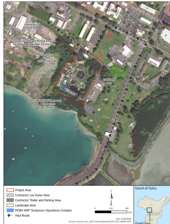
Figure 4. Proposed Construction Laydown Areas and Haul Routes.
