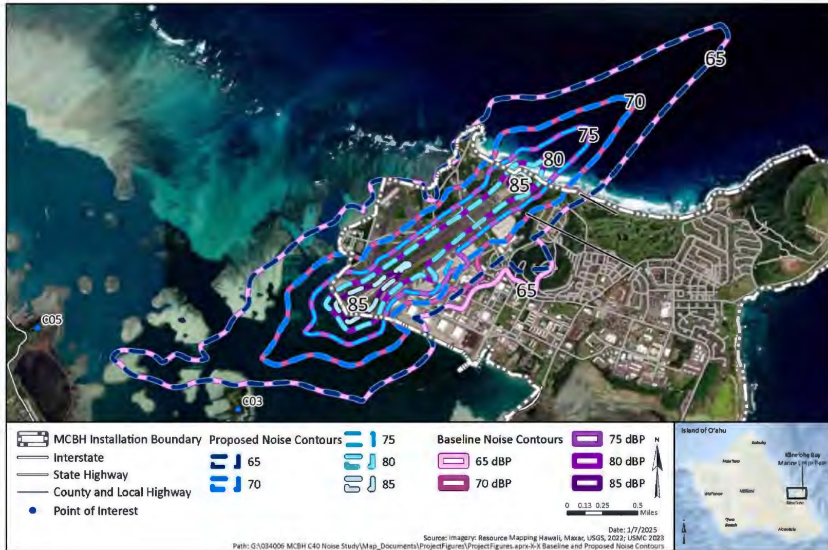
Figure 4-1 Proposed Action DNL Noise Contours and Points of Interest in the Vicinity of MCBH Kaneohe Bay
