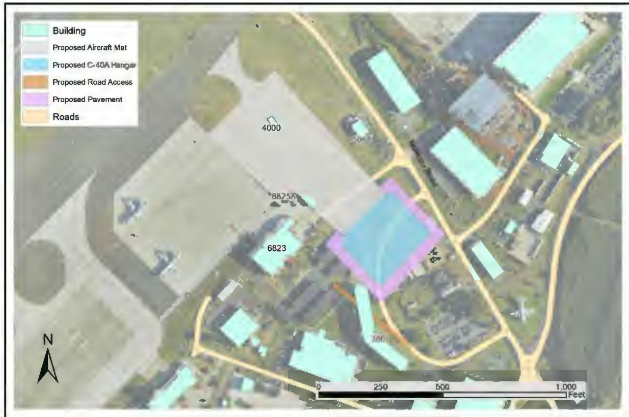
Figure 2-4. Proposed Hangar and Mat Layout at the Green Field Site
